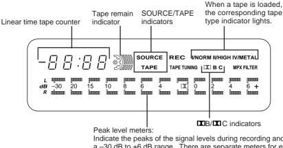
Indicate the peaks of the signal levels during recording and playback over a -30 dB to +6 dB range. There are separate meters for each left and right channel. These level meters have a peak hold function which holds the peak level for about 1.5 seconds. (The peak hold function works in the level from -10 dB to +6 dB.)
